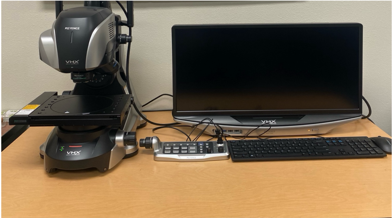
Figure 11: Keyence VHX 7000 Series Digital Microscope used for surface area measurement
