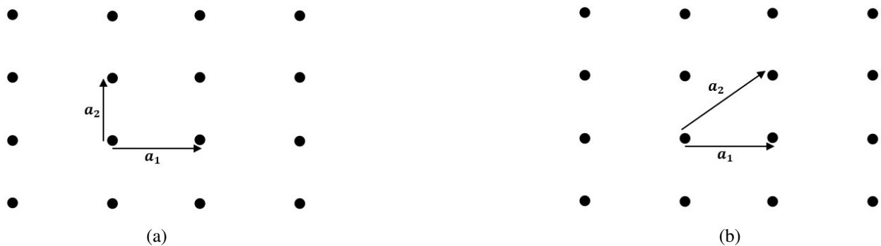
Figure 3.1: Primitive lattice vectors for (a) square and (b) oblique lattice in two dimension.
