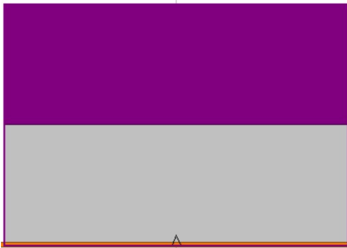
Figure 5.1: Two dimensional homogeneous dielectric medium. The lower rectangle (gray color) is the first dielectric medium, n_1 = 1.0 and upper rectangle (magenta color) represents the second dielectric medium, n_2 = 1.52 .
